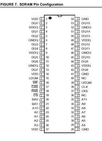
**Note:** To use the SDRAM, apply inverted clock from FPGA to the SDRAM for the proper SDRAM operations.
