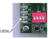
**D8** is Configuration Done LED that indicates successful completion of downloading process. The CONFIG\_DONE pin (**U11.145**) of the Cyclone device controls this LED.
