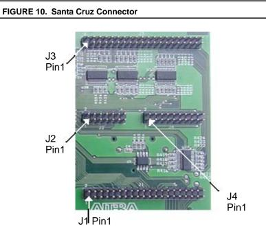
Figure 11, Figure 12, Figure 13 & Figure 14 show the pin description of the connectors J1, J2, J3 & J4 respectively.
